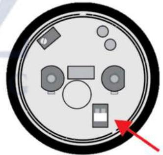
Make sure the switch heads towards the outside of the sensor.
